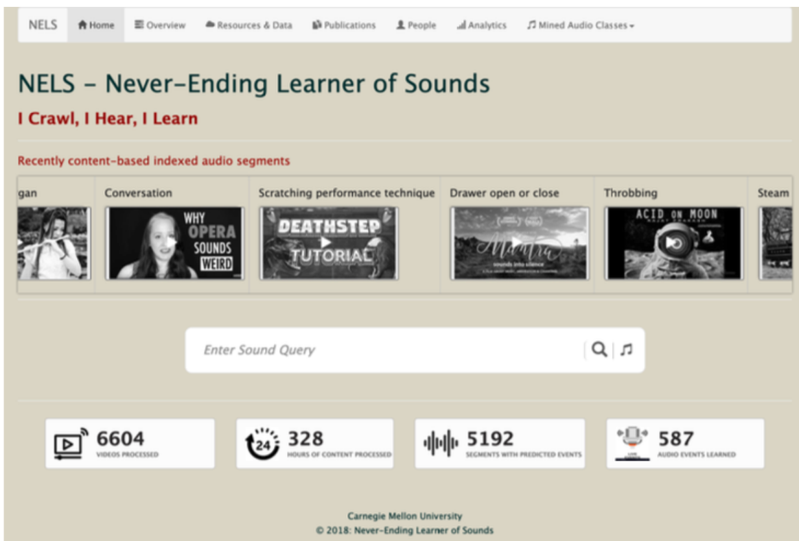
Figure 2.2: NELS user interface Interface: The user interface takes a text query and recovers audio recordings that best match the text in the indexed database.
